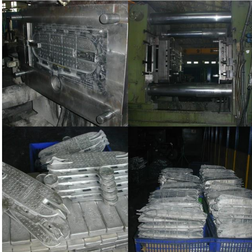
Exhibit 8-8. Production of the Mg deck requires a die (or mold) as shown in the upper two panels. The raw castings as they come from the die are shown in the lower two panels. The lower right panel shows a production batch of about 500 pieces.
