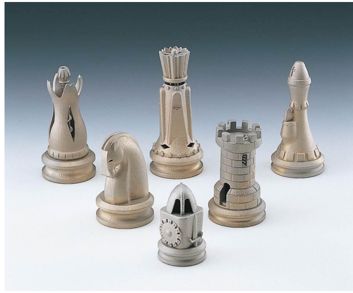
Exhibit 5-6. Chess pieces fabricated using the selective laser sintering (SLS) process, a rapid prototyping technology. Source: http://www.kinzoku.co.jp/image/zoukei_p3_b.jpg .
