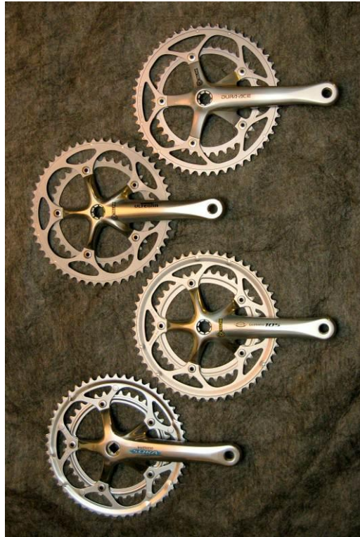
Exhibit 8-4. Shimano bicycle cranks are available in several different quality levels for a given size and application type. These four artifacts are all 170 mm 53/39-tooth cranks sold by Shimano at prices from $60 (bottom) to $350 (top). This is an example of quality variety.
