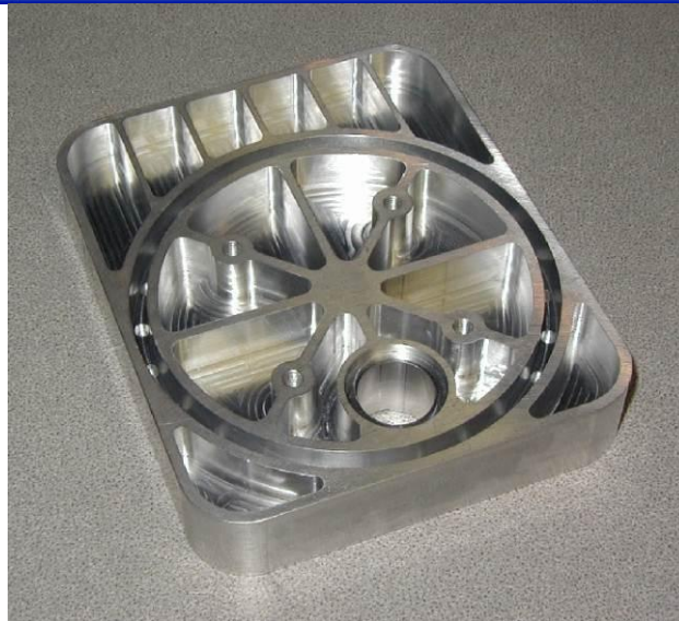
Exhibit 5-7. Aluminum part flexibly produced by a CNC milling machine. A web-based design program can be used to create instructions for the milling machine. Source: emachineshop.com.
